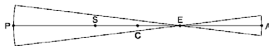
Fig. 35. At the apsides, the velocity of the planet is inversely proportional to the distance to the Sun
